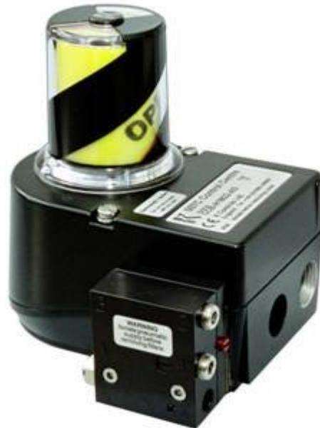
When the override is on a pilot solenoid within a top mounted integrated device, a deliberate act of cover removal would need to precede manual operation. If speed control is required this is best achieved by fitting a needle valve to each exhaust port (not inlet) of the pilot valve.
