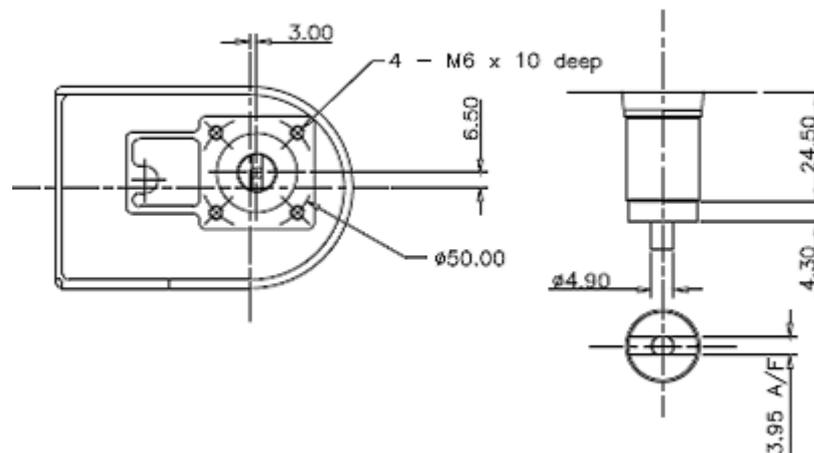
**VDI/VDE 3847** is a relatively recent standard that defines the standardised mechanical and pneumatic interface between a positioner and a linear actuator. This interface allows pipeless mounting and positioners that conform to this standard are interchangeable. The overall dimensions of the actuator and positioner are reduced and two point fixing allows the positioner to be fitted or replaced quickly.
